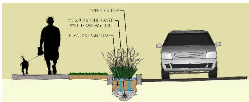
Figure 4-10. Typical Green Gutter Cross Section
